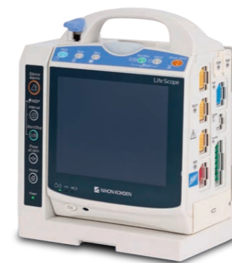
Transportmonitor Life Scope PT in separater DAU Data Acquisition Unit eindockbar.
